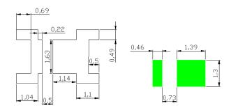
$\diamond$  Recommended solder pad design for heat dissipation (EMC T3C Series -3030)
