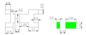
Recommended solder pad design for heat dissipation (EMC T34 Series -3020)
